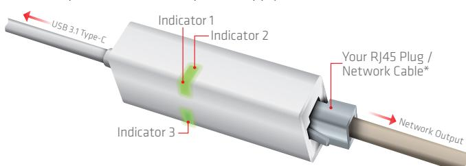
**Indicator 1:** this indicator turns **Green** to indicate **connection establishment** between host PC and Ethernet source.
