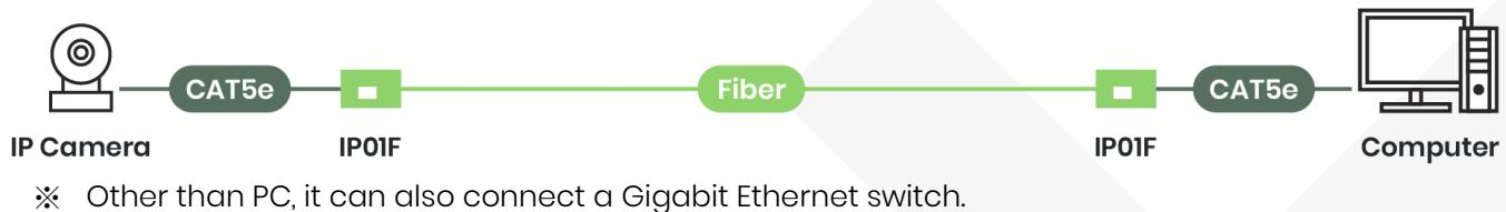
※ Other than PC, it can also connect a Gigabit Ethernet switch.
