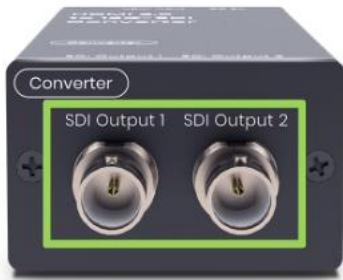
SDI02E-12G is equipped with two 12G-SDI output ports, allowing for simultaneous transmission of converted video signals to multiple SDI-compatible devices. These SDI output ports provide flexibility in signal routing and distribution, catering to various production and broadcasting setups.
